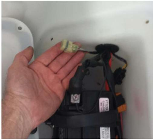
Remove the cover on the diagnostics connector by lifting the little tang, and pull the two halves apart. Route the Power connector (with Purple wire) to the front of the ski, through the front panel opening. Attach the power connector to the diagnostic connector.
