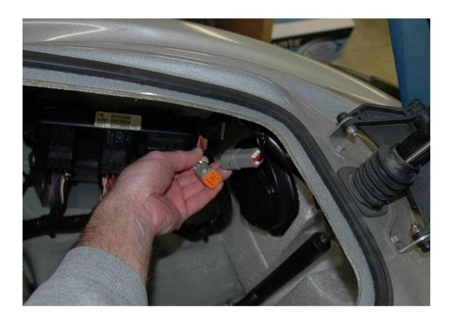
NOTE: Always remember to put the cap back on the diagnostic connector when you are finished with a Candoopro session! Otherwise your Maint light will be on and stay on!
