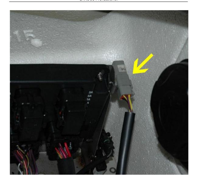
Disconnect the 6-pin connector from the sealing cap:
