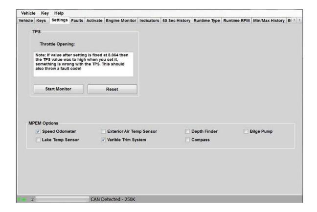
To Reset Throttle Position Sensor (TPS) on 2002-2011 models with Siemens ECU (non-iControl watercraft):
