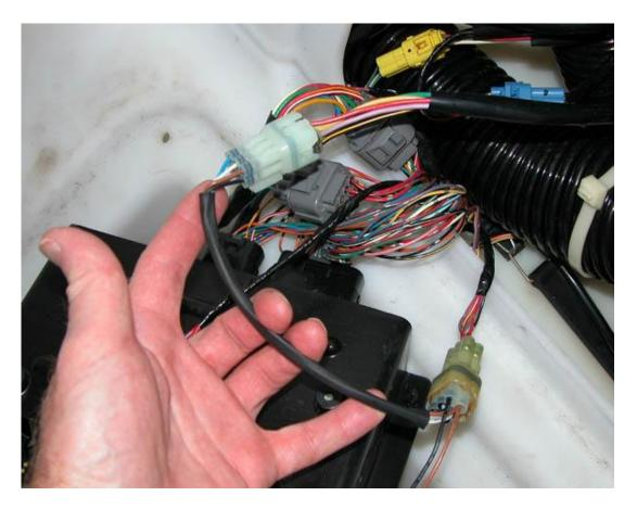
6. Once the Immobilizer Bypass cable is installed, connect the two small white one-pin connectors together on this cable:
