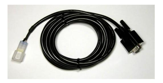
The 2010+ Adapter is used to connect the Main Diagnostic cable to the new-style connector on 2010+ Ultra skis:
