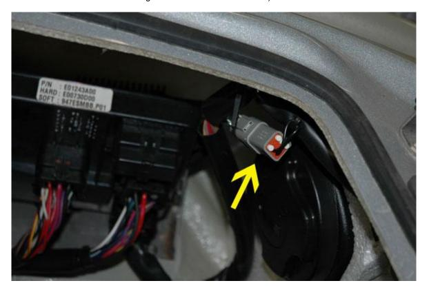
Disconnect the 6-pin connector from the sealing cap:
