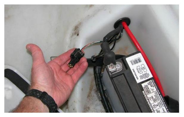
2. Remove the dust cap from the connector, and attach the Main Diagnostic cable to the diagnostic connector. NOTE: On 2007-2009 models, the Main cable connects directly to the connector on the ski. On 2010 models, you must first attach the 2010+ Adapter cable to the Main cable, then connect the 2010+ Adapter cable to the diagnostic connector on the ski.
