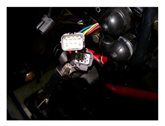
4. Disconnect the Main Relay connector and connect the Early Relay Bypass cable inline between the two halves of the Main Relay connector. Fasten the ring terminal of the Early Relay Bypass cable to the negative/ground (-) post of the battery:
