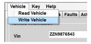
After you select Write, a popup box will instruct you to remove the key and wait until the connect light is off to complete the write operation.
