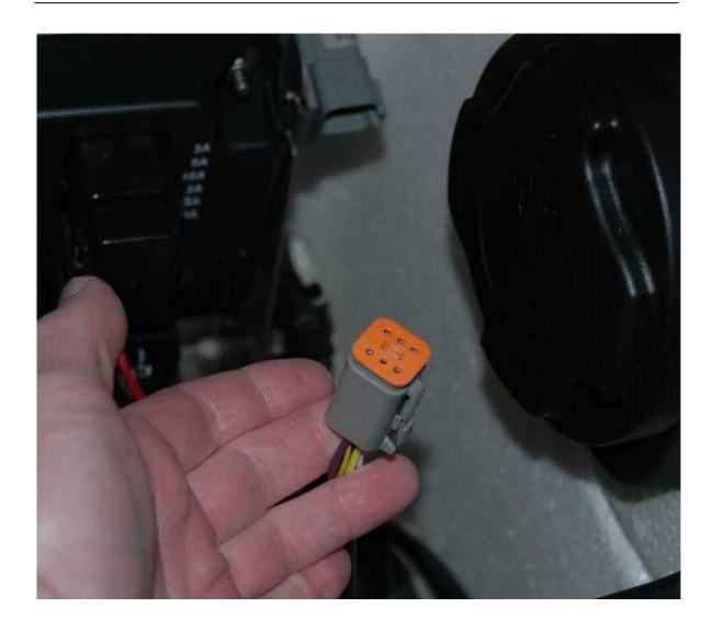
Warning: Always remember to put the cap back on the diagnostic connector when you are finished with a Candoopro session! Otherwise your Maint light will turn on and stay on!
