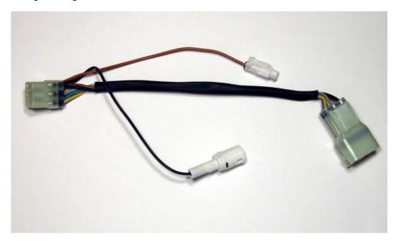
The 2-stroke DI Main Diagnostic cable is used to connect the Candoopro diagnostic box to the 1999-2003 STX-1100 Ultra 130 DI models :
