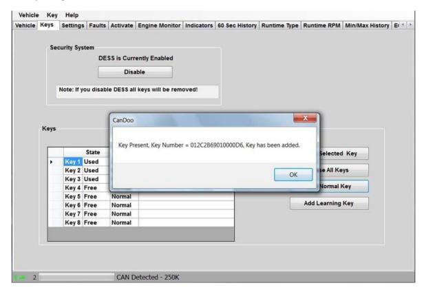
NOTE: If a key is not on the post, is not properly seated on the post, or is not a good key, you will see an error message "Key Not Found".
