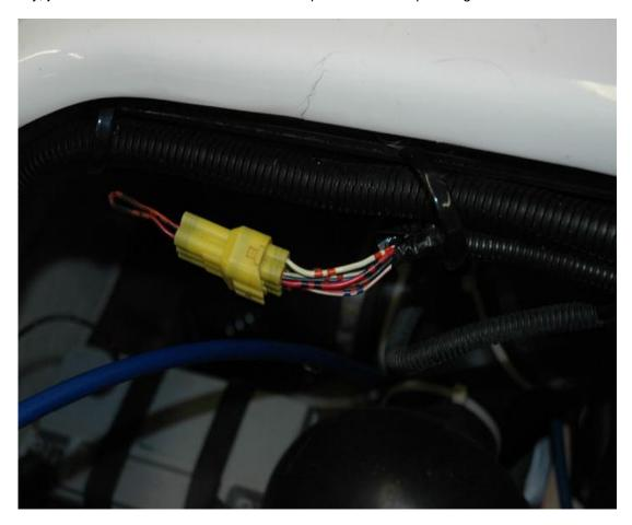
2. Remove the dust cap from the diagnostic connector, and attach the STX-1100 DI Main Diagnostic cable to the yellow diagnostic connector on the ski.
