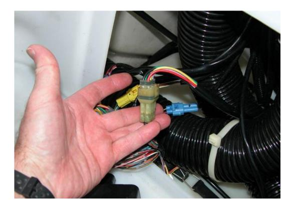
5. Disconnect this connector and connect the Late Immobilizer Bypass cable in-line:
