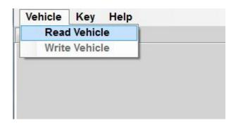
The CANDooPro system will now read the information from the MPEM. On most DESS skis, you will also hear a series of beeps from the buzzer during the transfer of data.
