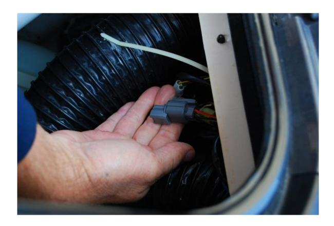
Disconnect this connector, and plug the Candoopro Yamaha adapter cable light gray connector into the mating connector on the Waverunner harness:
