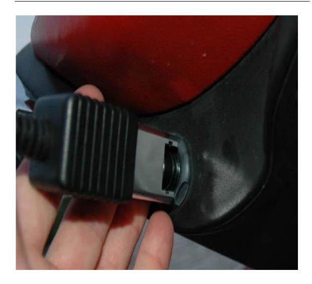
The DESS Adapter contains a magnet, which closes the reed switch in the DESS post, and turns on the MPEM. The MPEM should start communcating with the CANDooPro system. Once the CANDooPro system detects communcation with the MPEM, it should indicate that it is talking to the MPEM by a change in the status bar on the lower left of the screen.
