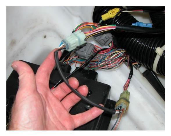
6. Once the Immobilizer Bypass cable is installed, connect the two small white one-pin connectors together on this cable:
