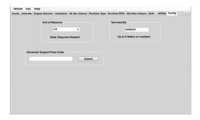
The **Config** tab allows you to change the overall program numbering system between US and Metric values, as well as allowing you to personalize the "**Serviced By** " setting.
