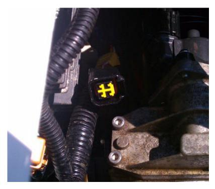
2. Remove the dust cap, and plug the Candoopro Kawasaki Main Diagnostic cable into this connector.
