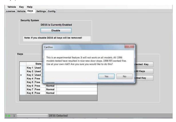
Simply select **Yes**, and the write the information to the MPEM by selecting **Vehicle** and **Write Vehicle**.
