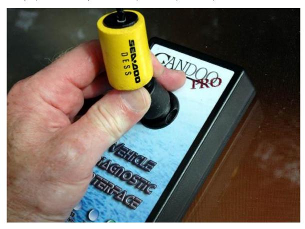
Once the key is on the post, click the type of key you wish to add. For example to add a normal key, click the "Add Normal Key" button. A box will appear indicating the key has been added to the key listing.
