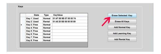
Now that the key has been deleted, you must Write this change into the MPEM. Select "Vehicle" in the upper tab, then "Write Vehicle".
