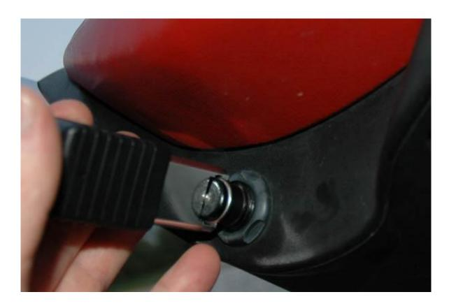
Slide the DESS adapter over the DESS post as shown below, with a quick motion. You
