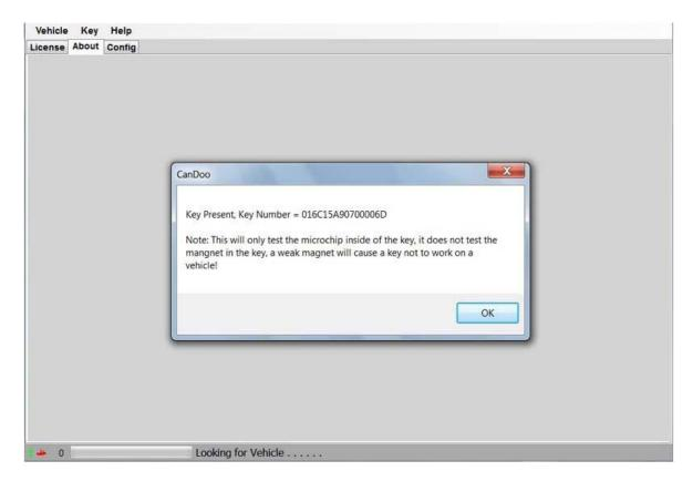
The key number shown by the popup box is the 64 bit serial number of the key. (Shown in Hexidecimal format) Note that this only tests the microchip in the key; it does not check for a weak magnet.
