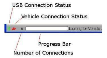
• Connect the Candoopro system to the Waverunner diagnostic connector.
