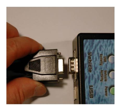
2. Connect the DESS post adapter cable to the 9pin/6-pin cable, by sliding the two cables together until they click..
