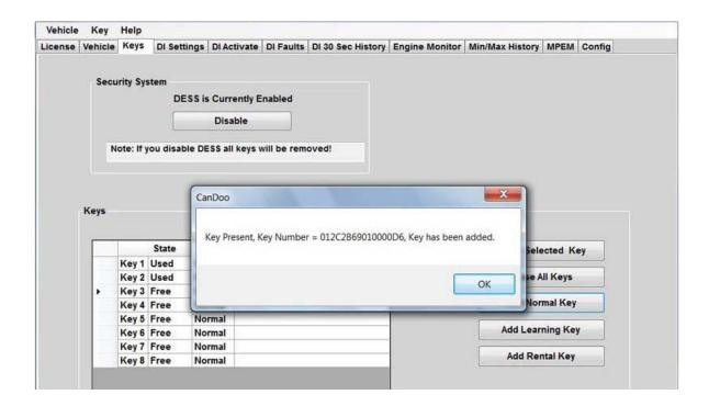
NOTE: If a key is not on the post, is not properly seated on the post, or is not a good key, you will see an error message "Key Not Found".
