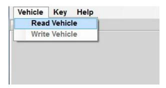
The Candoopro system will read the data from the ECU. You are now ready to read and clear faults, view operating history, and activate various functions available for that particular model.
