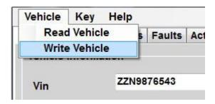
After you select Write, a popup box will instruct you to remove the key and wait until the connect light is off to complete the write operation. (a box will not popup on 2009 and newer models with the iControl system; you do not need to remove the key on these models) Follow the instructions in the box, and especially take note that on 2007 and newer models, you need to take the key off, put it back on, then remove again to complete the write operation.
