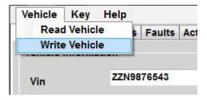
After you select Write, a popup box will instruct you to remove the key and wait until the connect light is off to complete the write operation.
