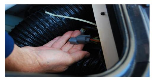
2. Disconnect this connector, and plug the Candoopro Yamaha adapter cable light gray connector into the mating connector on the Waverunner harness:
