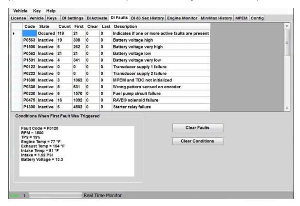
As you can see, there are many faults with counts in the table above! This is very common to see; many faults in the Count column, which have continued to build up over the years. Plus, the faults have never been cleared since the ski was new! Please refer to the Fault Diagnosis for strategies on how to zero in on recent faults.
